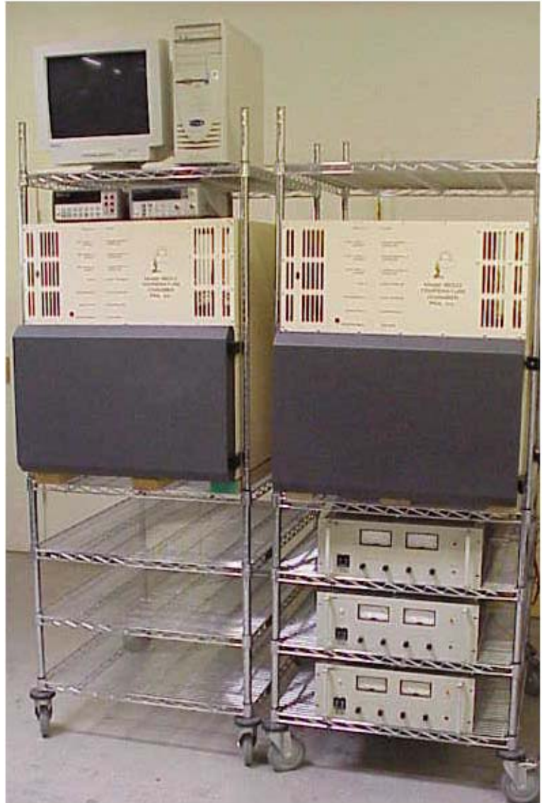
System shown on optional racks with one chamber having OCXO power supplies
