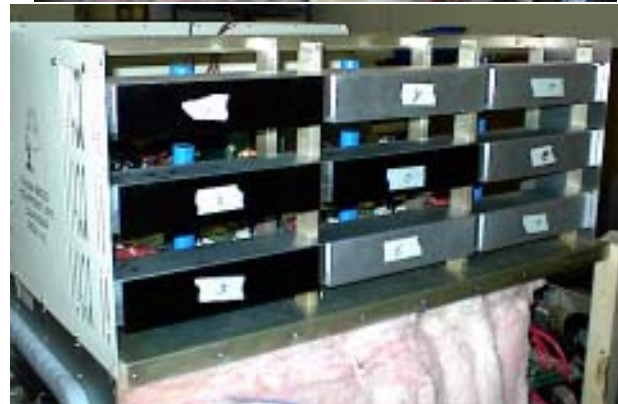
Power Supplies Chamber side removed, showing the 9 supplies and the air ducts and power supply heat sinks.
